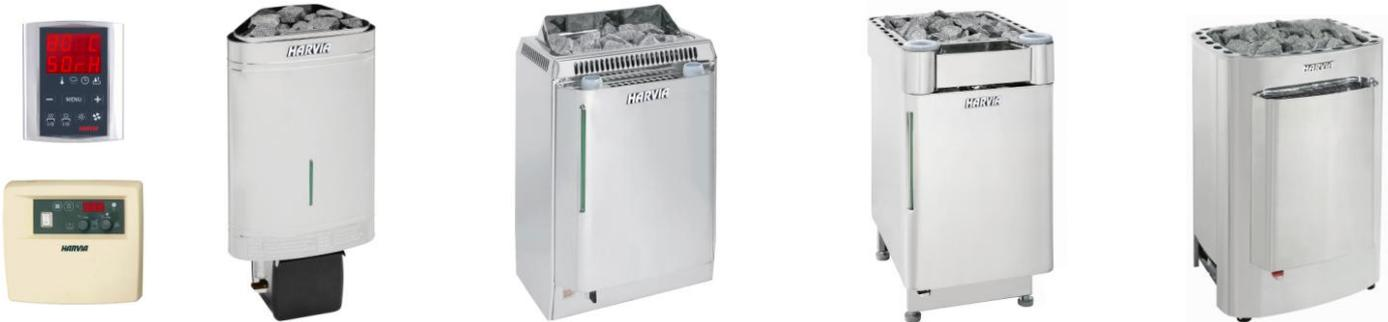
To achieve this particular environment (also called a tepidarium, calidarium, etc..) must be installed inside the sauna a BIO-HEATER, which is a traditional heater for sauna (with heating elements embedded in the rocks) to which it is built - in front - a steam generator (a water tank with an heating element inside).
