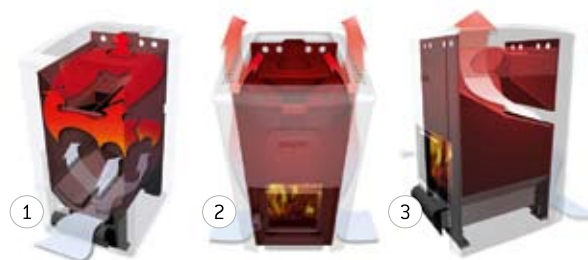
An example of the air and fire circulation of a Harvia stove 1. Incoming air and fire circulation during the burning process. 2. Air heating between the body and the outer casing. 3. Air flow through the stone space.
